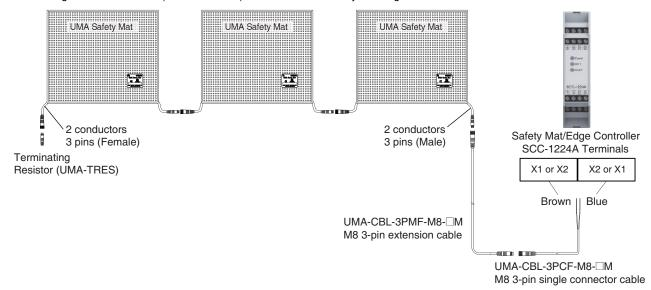
• Connecting three 2-cable Mats (UM \( \subseteq A-\subseteq -2) to a MC3 Safety Mat Controller.
