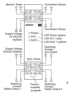
\* Remove the factory-installed jumper between terminals 14 and 23 if safety outputs 1 and 2 are not connected in series.
