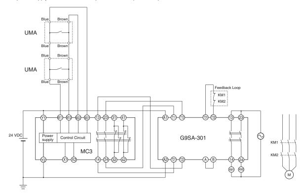
KM1, KM2: Magnetic contactor M: Motor
