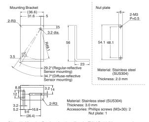
\*Use this Mounting Bracket when installing the ZX2-LD100 (L) as a normal Diffuse-reflective or Regular-reflective Sensor Head.
