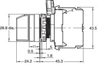
Two-notch Switches with Metal Bezels A22N□-2M□
