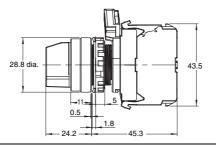
Three-notch Switches with Plastic Bezels A22N□-3B□
